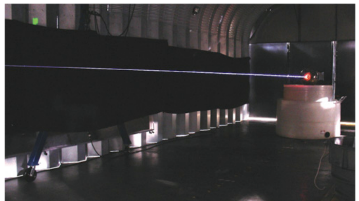
Ionatron's prototype weapon uses laser light to ionize the air and channel a high-voltage electric discharge, which could be adjusted to disable a person without killing. Ionatron
