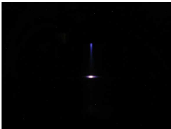
Fig. 2. Welder electron beam propagating in atmosphere after exiting the plasma window.
