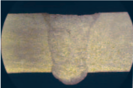
A complete penetration weld in 0.125-in.-thick 316 stainless steel at a travel speed of 15 in./min at 3 kW of power.
