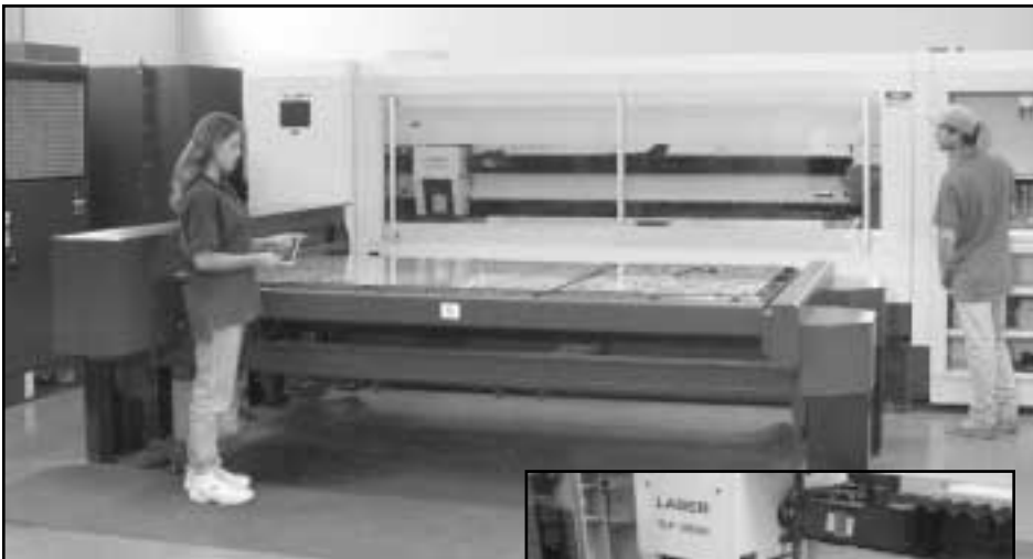
Above: The TRUMPF L 2530 is Acceleron's first flat pattern high-volume production cutting machine. Right: Cut edge quality, accuracy and repeatability were the key benefits offered by TRUMPF
