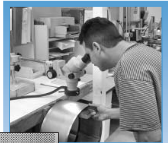
Above: Spot inspection of drilled components is a critical function in maintaining accurate hole diameter criteria.
