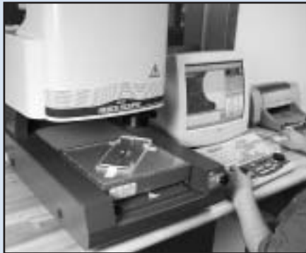
The Quick Scope is becoming an invaluable part of Acceleron's inspection process.
